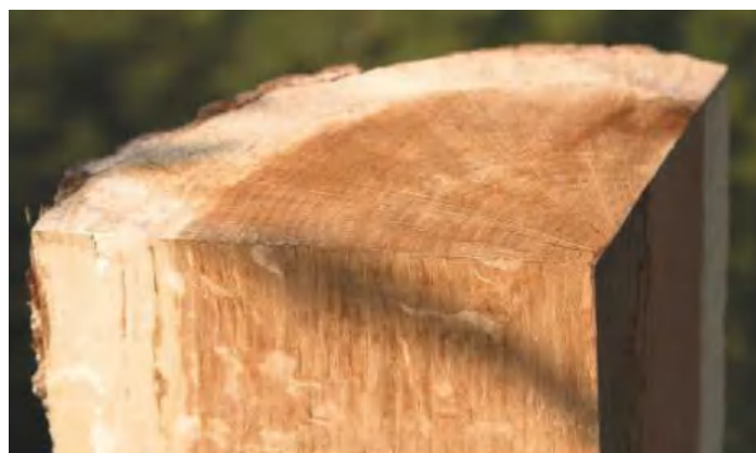
▲ Pic.5 This oak log has been cut into quarters so you can see the rays running between the centre and outside of the trunk as well as the fibres running from top to bottom
